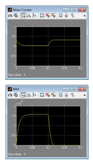
2 Run the simulation. Note the effect of reduced voltage on the no-load speed.
