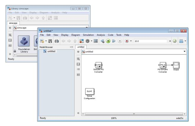
By default, the model name is not specified, the model contains a Solver Configuration block with the default solver set to ode15s, a Simulink-PS
